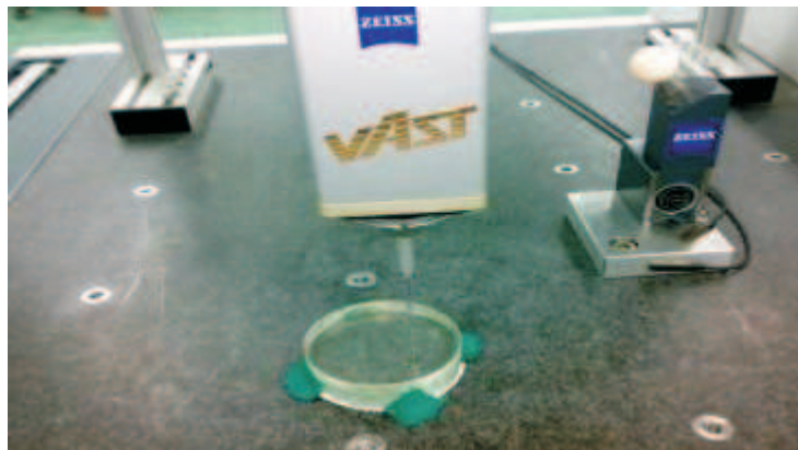
Fig. 2. Flatness measurements of the optical flat are realized by the Zeiss CMM using probing – scanning head Zeiss Vast.
