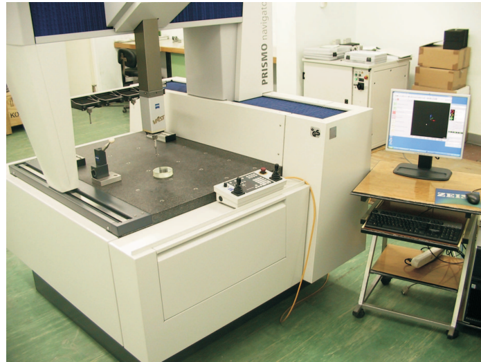
Fig. 1. The alignment process of the optical flat is on the CMM's table.
